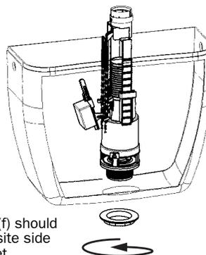
**NB:** The small float (f) should be on the opposite side to the water inlet.
